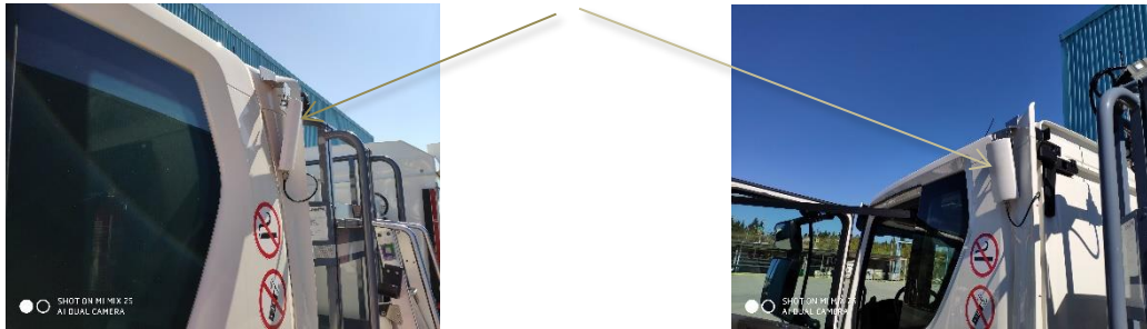
Sector antenna with installation bracket.
