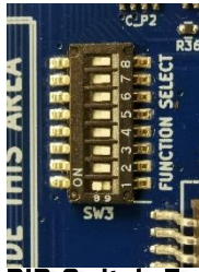
SW3, DIP Switch Function select (See chapter 2.10)
